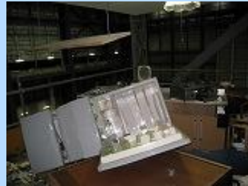
Figure 2-1 Result of shaking table test on room contents (from 01, 2008 test)
