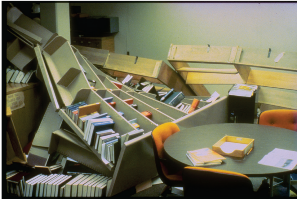
Figure 6.5.2.1-1 Failure of poorly anchored wood and metal book shelves at the Lawrence Livermore Laboratory, Livermore, California (NGDC, 2009).
