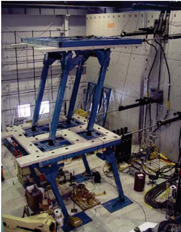
Figure 6.3.2.2-5 Two-story nonstructural component simulator at the University of Buffalo, SUNY shown at left. Preparation for dynamic testing of stud partitions for the NEES Nonstructural Project shown at right. Tests such as these improve understanding of the seismic behavior of nonstructural components (Photos courtesy of University of Buffalo, SUNY).
