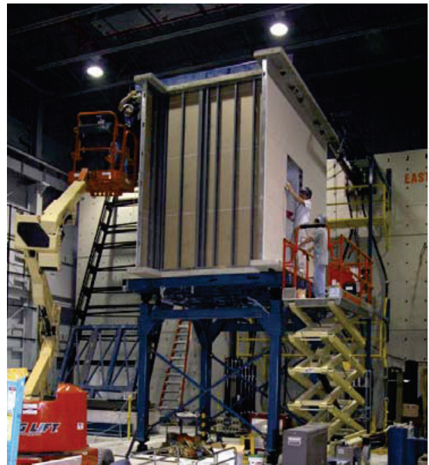
Figure 6.3.2.2-5 Two-story nonstructural component simulator at the University of Buffalo, SUNY shown at left. Preparation for dynamic testing of stud partitions for the NEES Nonstructural Project shown at right. Tests such as these improve understanding of the seismic behavior of nonstructural components (Photos courtesy of University of Buffalo, SUNY).
