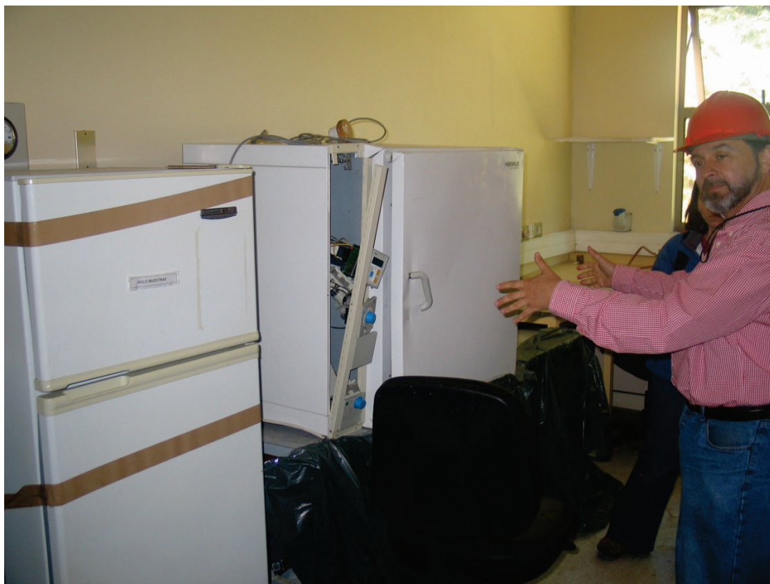
Figure 6.5.6.2-1 Incubator in the microbiology lab at the University of Concepción was ruined in the 2010 magnitude-8.8 Chile Earthquake (Photo courtesy of Bill Holmes, Rutherford & Chekene).
