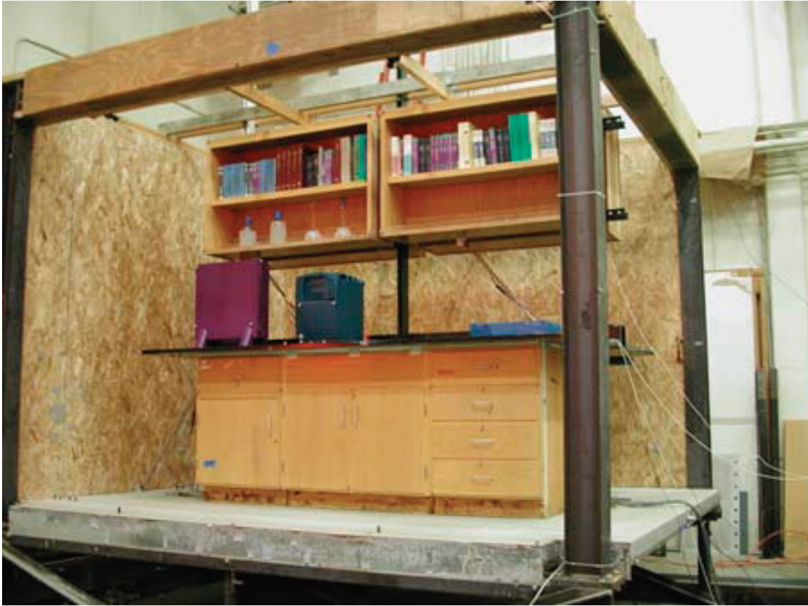
Figure 6.5.6.2-2 Set-up for shake table testing at UC Irvine of typical laboratory bench and shelving with countertop equipment and shelved books and supplies. Testing was done in order to develop fragility curves for use in developing performance based design parameters (PEER Testbed Study on a Laboratory Building: Exercising Seismic Performance Assessment; Comerio, Editor. PEER 2005/12).
